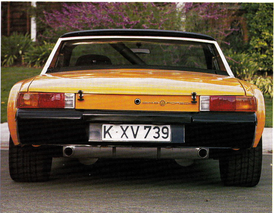
■ Below —The Kinsts’ 914-6 now wears factory steel GT flares and proper fiberglass GT decklids.
